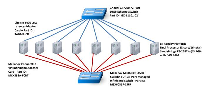
The testbed used in the benchmarks consists of a number of servers dual connected to a 10Gbps Ethernet network and to the latest FDR IB fabric. Identical tests were run using the two fabrics for an objective comparison. On the Ethernet side, the tests were conducted using simple NIC attachment (stateless offload), TOE (TCP/IP full offload) and iWARP.
