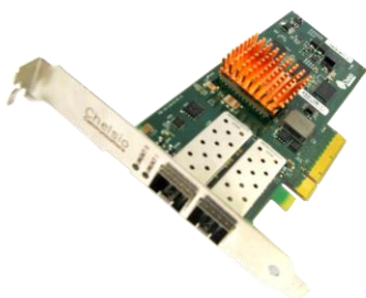
Figure 1 – The high-performance, dual-port Chelsio T420-LL-CR 10GbE Unified Wire Adapter
