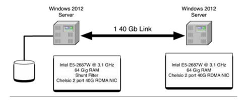
**Network configuration:** Two Microsoft Windows Server 2012 machines connected back to back using a pair of Chelsio 2-port adapters. One 40G port is used. The port on the server is configured as 102.50.50.x/24.
