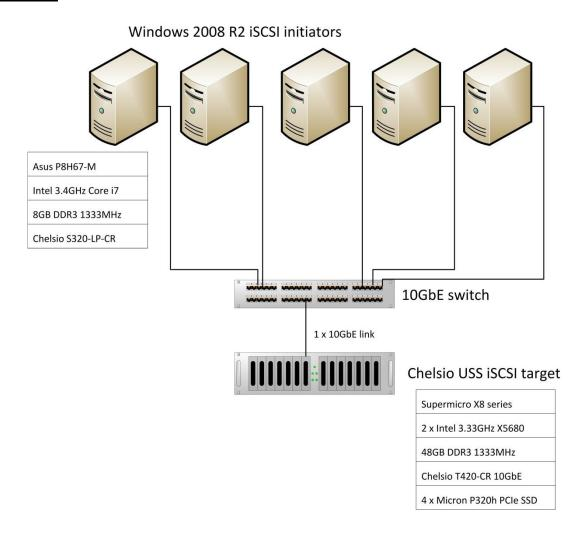
**Network configuration:** Five iSCSI initiator systems are connected to the 10GbE switch via port 0 of a Chelsio S320-LP-CR 10GbE adapter on each system with Twinax cables. The USS iSCSI target system is connected to the 10GbE switch via port 0 of a Chelsio T420-CR 10GbE adapter.
