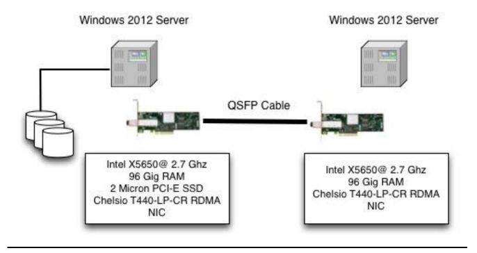
**Network configuration:** Two Microsoft Windows Server 2012 machines connected back to back using a pair of Chelsio T440-LP-CR 4-port adapters and a single QSFP cable. All 4 available ports are utilized.
