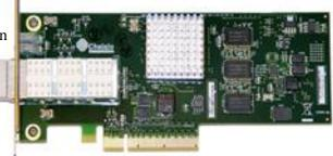
board hardware that off-loads TCP/IP, iSCSI, FCoE and iWARP RDMA processing from its host system.
