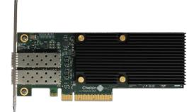
The fifth-generation (T5) technology from Chelsio provides the highest 10GbE performance in the industry and dramatically lowers host-system CPU communications overhead with on-board hardware that offloads TCP/IP, iSCSI, FCoE and iWARP RDMA processing from the host system and frees up host CPU cycles for other applications. As a result, the system benefits from higher bandwidth, lower latency, and reduced power consumption.
