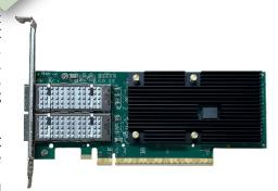
communications. Thanks to an on-board hardware, that offloads TCP/IP, UDP/IP, Unified RDMA (RoCEv2 and iWARP), iSCSI, NVMe-oF, NVMe/TCP, NVGRE, VXLAN, and TLS/IPsec processing from its host system and frees up host CPU cycles for the user applications. As a result, the system has the benefits of higher bandwidth. lower latency, and reduced power consumption.
