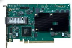
communications overhead thanks to on-board hardware that offloads TCP/IP, UDP/IP, Unified RDMA (RoCEv2 and iWARP), iSCSI, NVMe-oF, NVMe/TCP, NVGRE, VXLAN and TLS/IPsec processing from its host system and frees up the host CPU cycles for the user applications. As a result, the system benefits from higher bandwidth, lower latency, and reduced power consumption.
