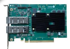
communications overhead thanks to on-board hardware that offloads TCP/IP, UDP/IP, Unified RDMA (RoCEv2 and iWARP), iSCSI, NVMe-oF, NVMe/TCP, NVGRE, VXLAN, and TLS/IPsec processing from its host system and reduces the host CPU cycles for the user applications. As a result, the system benefits from higher bandwidth, lower latency, and reduced power consumption.
