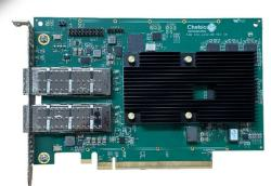
communications overhead thanks to on-board hardware that offloads TCP/IP, UDP/IP, Unified RDMA (RoCEv2 and iWARP), iSCSI, NVMe-oF, NVMe/TCP, NVGRE, VXLAN and TLS/IPsec processing from its host system and frees up the host CPU cycles for the user applications. As a result, the system benefits from higher bandwidth, lower latency, and reduced power consumption.
