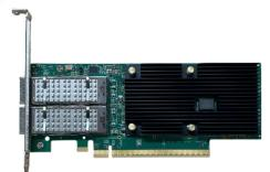
communications overhead thanks to on-board hardware that offloads TCP/IP, UDP/IP, Unified RDMA (RoCEv2 and iWARP), iSCSI, NVMe-oF, NVMe/TCP, NVGRE, VXLAN, and TLS/IPsec processing from its host system and frees up the host CPU cycles for the user applications. As a result, the system benefits from higher bandwidth, lower latency, and reduced power consumption.
