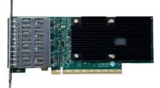
communications overhead thanks to on-board hardware that offloads TCP/IP, UDP/IP, Unified RDMA (RoCEv2 and iWARP), iSCSI, NVMe-oF, NVMe/TCP, NVGRE, VXLAN, and TLS/IPsec processing from its host system and reduces the host CPU cycles for the user applications. As a result, the system benefits from higher bandwidth, lower latency, and reduced power consumption.
