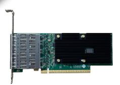
hardware, that offloads TCP/IP, UDP/IP, Unified RDMA (RoCEv2 and iWARP), iSCSI, NVMe-oF, NVMe/TCP, NVGRE, VXLAN, and TLS/IPsec processing from its host system and frees up host CPU cycles for the user applications. As a result, the system has the benefits of higher bandwidth, lower latency, and reduced power consumption.
