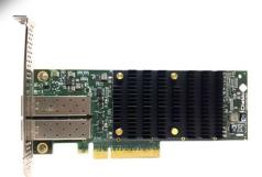
hardware, that offloads TCP/IP, UDP/IP, Unified RDMA (RoCEv2 and iWARP), iSCSI, NVMe-oF, NVMe/TCP, NVGRE, VXLAN, and TLS/IPsec processing from its host system and frees up host CPU cycles for the user applications. As a result, the system has the benefits of higher bandwidth, lower latency, and reduced power consumption.
