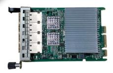
communications. Thanks to an on-board hardware, that offloads TCP/IP, UDP/IP, Unified RDMA (RoCEv2 and iWARP), iSCSI, NVMe-oF, NVMe/TCP, NVGRE, VXLAN, and TLS/IPsec processing from its host system and frees up host CPU cycles for the user applications. As a result, the system has the benefits of higher bandwidth, lower latency, and reduced power consumption.
