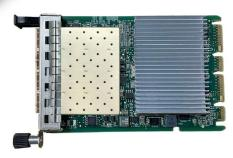
communications. Thanks to an on-board hardware, that offloads TCP/IP, UDP/IP, Unified RDMA (RoCEv2 and iWARP), iSCSI, NVMe-oF, NVMe/TCP, NVGRE, VXLAN, and TLS/IPsec processing from its host system and frees up host CPU cycles for the user applications. As a result, the system has the benefits of higher bandwidth, lower latency, and reduced power consumption.
