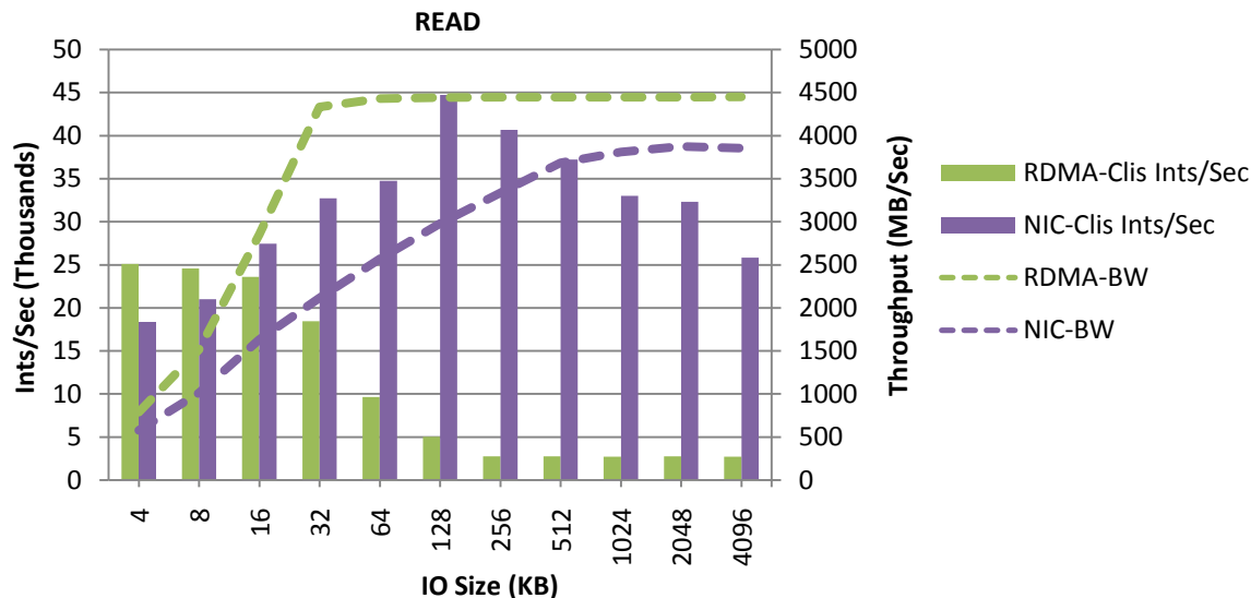
Figure 3 – NFS READ Throughput and Interrupts/sec vs. IO Size
