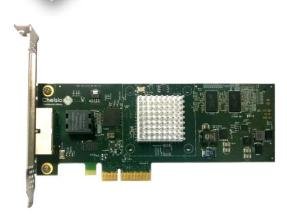
offloads TCP/IP, iSCSI, FCoE and iWARP RDMA processing from its host system. The T502-BT uses the same T5 engine that powers the 10G and 40G adapter versions. It supports the same complete suite of offloaded protocols, traffic management and rich server adapter feature set.
