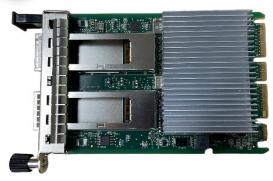
T62100-SO-OCP3 based on the sixth-generation (T6), server offload technology from Chelsio provides the highest performance and efficiency, sub micro-second end-to-end latency, dramatically lowers host system CPU communications overhead and frees up host CPU cycles for useful applications. This will enable savings in host CPU acquisition costs, power and operational costs, and dramatically increases system performance.
