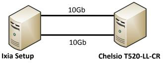
An Ixia setup running IxOS operating system version 5.30.450.31 and IxAutomate version 6.70.76.19, was connected back-to-back to a server with Chelsio's T520-LL-CR adapter. Chelsio Unified Wire software version 2.8.0.0 was installed on the server. The *RFC2544 Throughput* test was used to determine the line rate performance.
