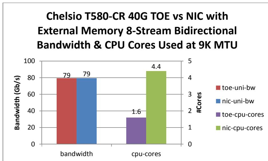
The graph above shows both the bandwidth achieved and CPU utilization for the offload (*TOE*) and NIC cases. While both can achieve line rate bidirectional transfer performance, the *TOE* frees up 3 cores that otherwise would have been wasted in network protocol stack processing. This effectively allows 75% more of the investment in processing to be reclaimed for useful applications.
