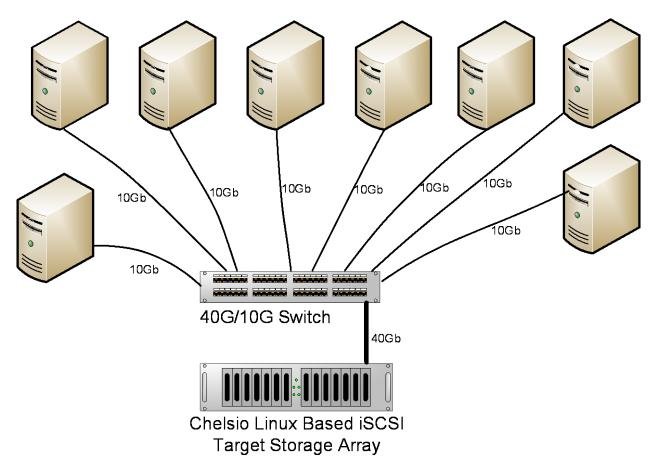
**Network configuration:** The network configuration consists of three components; the 40Gb/10Gb switch, the iSCSI target storage array with one 40Gb port, and eight iSCSI initiator peer machines running at 10Gb. End to end standard 1500 byte MTU Ethernet frames are used throughout.
