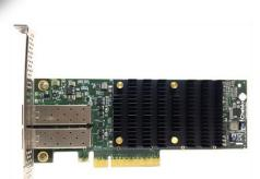
This adapter, based on the sixth-generation (T6), memory free technology from Chelsio, provides the highest performance and efficiency, dramatically lowers host-system CPU communications overhead and frees up host CPU cycles for useful applications. As a result, the system benefits from higher bandwidth, lower latency and reduced power consumption.
