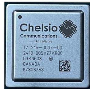
The seventh generation T7 ASIC technology from Chelsio provides the highest performance and efficiency, with dramatically lower host system CPU communications overhead. Thanks to on-board hardware, that offloads TCP/IP, UDP/IP, Unified RDMA (RoCEv2 & iWARP), iSCSI, NVMe-oF, NVMe/TCP, NVGRE, VXLAN, and TLS/IPsec processing from its host system and frees up host CPU cycles for user applications. As a result, the system benefits from higher bandwidth, lower latency, and reduced power consumption.
